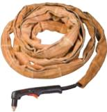
**Leather torch sheathing**Available in 25' (7.6 m) sections, this option provides additional protection for torch leads against burn-through and abrasion.
